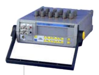
The SHP 101 bench top instrument is capable of scanning up to 12 temperature sensors. When used with the Precision Thermometer PHP 601, thermocouples and RTDs can be measured without loss of signal integrity or performance. Each block may be configured either as two measurement channels (thermocouple or voltage measurements) or as a 4 wire measurement (RTDs).
